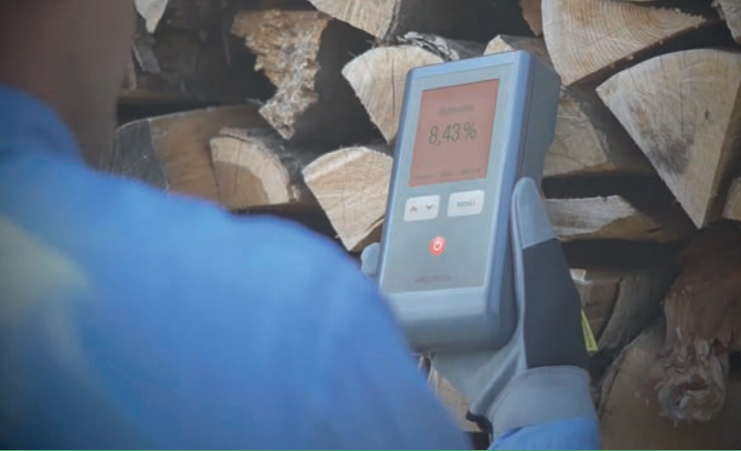
DATEC-COMPACT as a wood moisture measuring device
